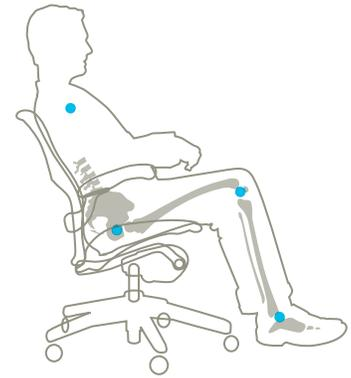
**Design Solution:** Provide support that nests the sacral-pelvic area and tilt action that echoes body mechanics.
